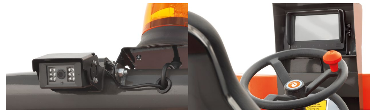
7. FULL VISIBILITY SYSTEM: Front and rear camera, TFT screen and obstacle detectors.
